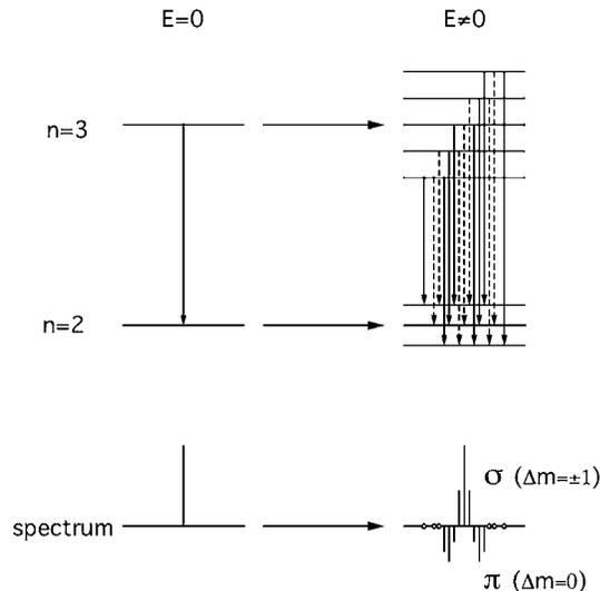
FIG. 1. Conceptual diagram of energy level change and spectral line splitting due to the Stark effect.
