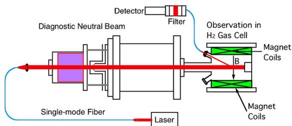
FIG. 3. MSE-LIF development laboratory setup.
