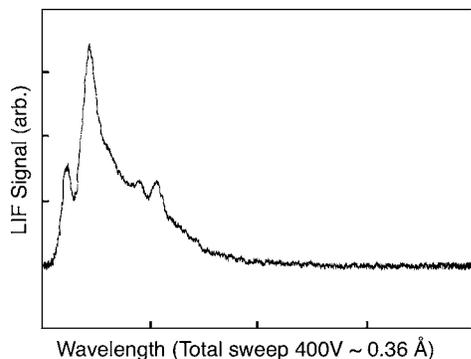
FIG. 5. Data in  $\sim 40$  G magnetic field showing asymmetry of line shapes.
