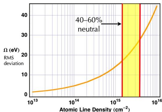
FIG. 4. Estimated beam straggling parameter vs line density for a proton beam in  $H_2$  gas.
