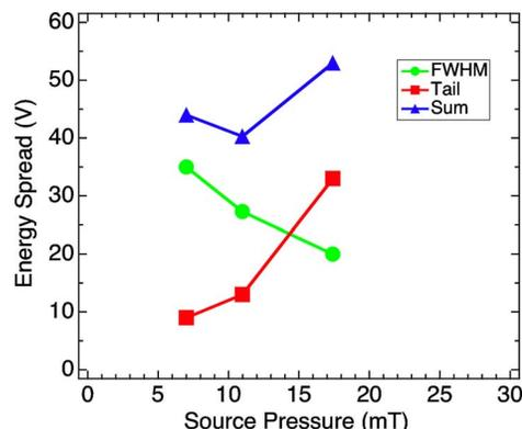
FIG. 6. Variation of neutral beam energy spread with the source operating pressure. Shown separately on the plot are the symmetric broadening (filled circles), asymmetric tail (filled squares), and the sum (filled triangles)
