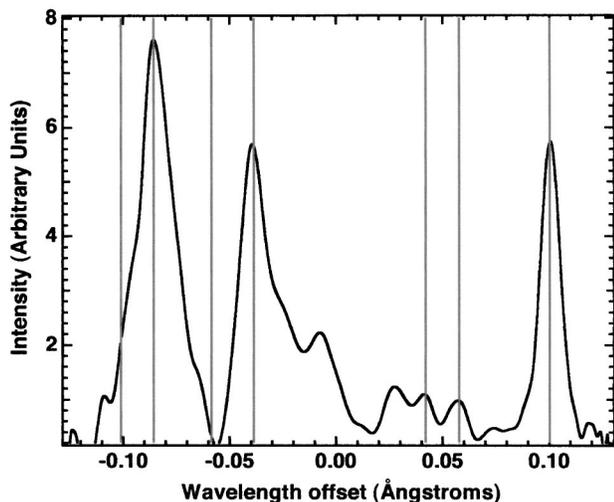
FIG. 2. LIF data of beam in neutral gas. Gray bars are Doppler-shifted Balmer- $\alpha$  fine structure line locations.
