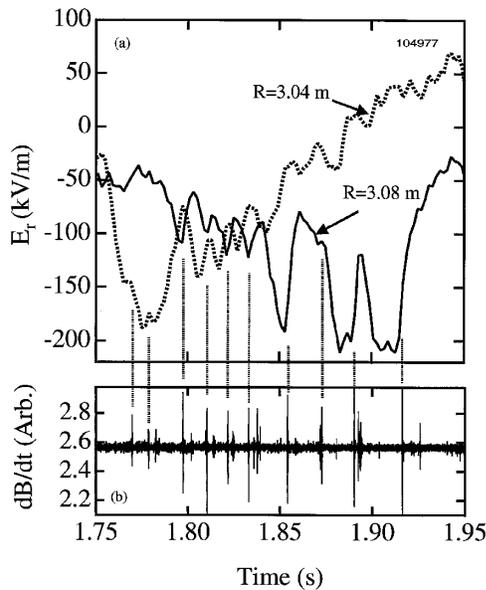
FIG. 5. (a) The time evolution of  $E_r$  at two radii and (b) Mirnov coil signal with MHD bursts correlated with changing  $E_r$ .
