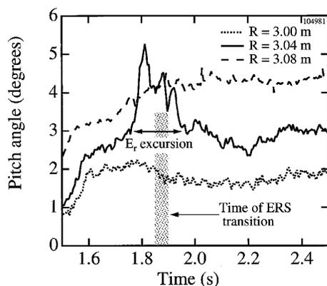
FIG. 3. The magnetic field pitch angle evolution of three sight lines. The time of the ERS transition is at 1.85–1.90 s.
