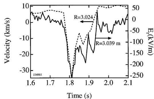
FIG. 4. The time evolution of  $E_r$  (solid line) from MSE and the measured poloidal rotation velocity (dashed line) at similar radii.
