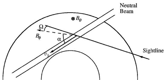
FIG. 1. Viewing geometry for the MSE diagnostic and neutral beam on TFTR. Twenty sight lines cover from inboard of the magnetic axis to the outboard plasma edge.
